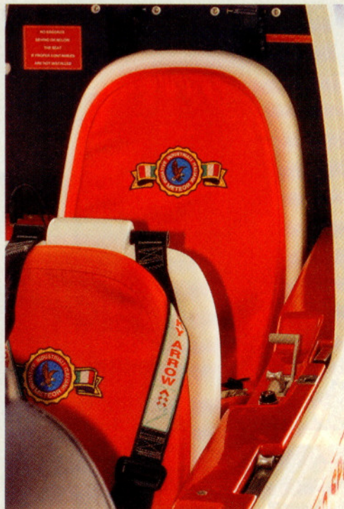
To get to the engine the pilot lowers the tail, but checking the oil requires a climb using the back seat. The rear seat (right) pulls forward to reveal a storage area, but pack lightly.
